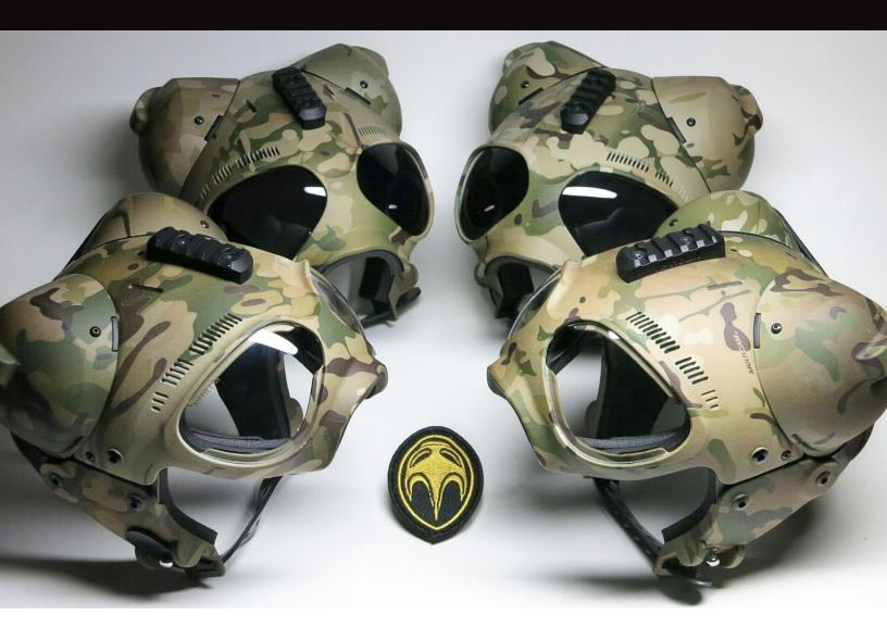
Nylon helmet shells are prepped with an epoxy primer and color coat. Then, the multicam pattern is applied using a hydro-dipping process. Finally, the parts are sprayed with a matte urethane clear coat. The vendor offering this service has an average lead time of 3-4 weeks.
